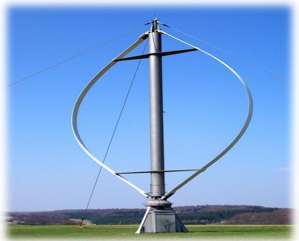
Figura 2 - Turbina eolica Darrieus
