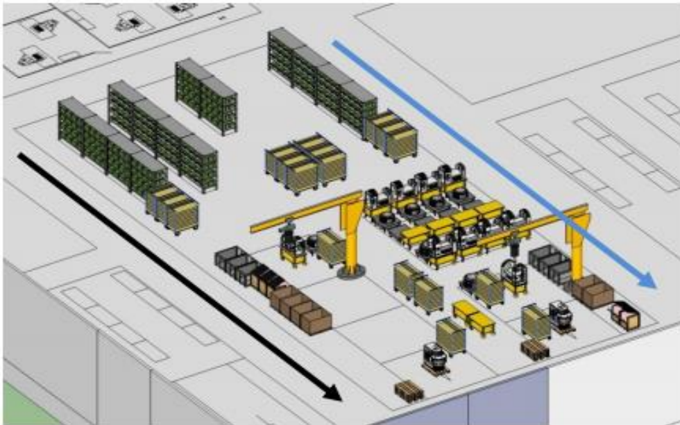
Fig. represent the diagram of the final layout of the pilot channel with two assembly lines and their respective supermarkets.
