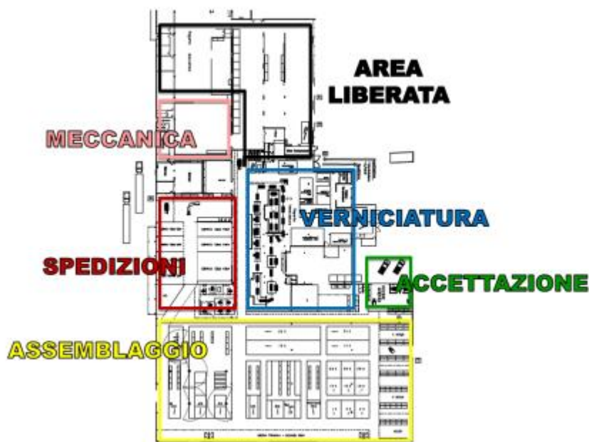
Fig. rappresent the factory layout after Kaizen shipyard
