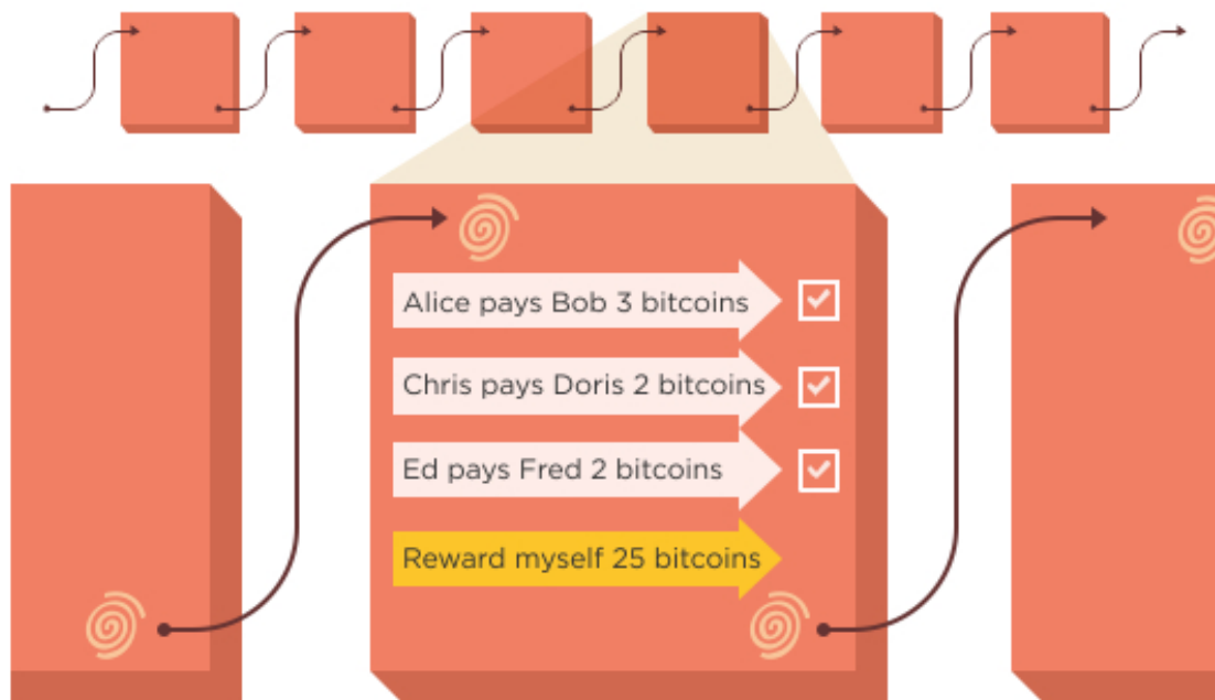
Figure 1.1: A Chain of Blocks Linked Together By Hash 'Fingerprints' [4]
