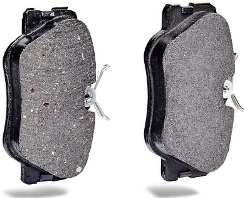
Figura 3.9 “Brake pads after stress test: Counterfeit (left) and original (right).” Fonte: Mercedes<sup>127</sup>
