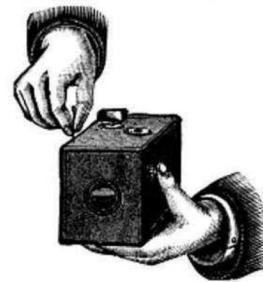
Fig. 1.—Setting the Shutter.
