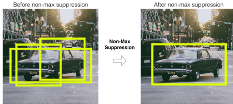
Figure 1.7: The effect of Non-Max Suppression in Object detection using YOLO [5]
