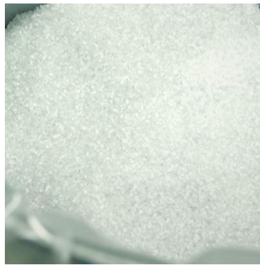
Image 1.3.2 - Luxottica's Plastic Lenses production presentation (2022). "Polyamide granules". Leonardo, Science for a new Vision
