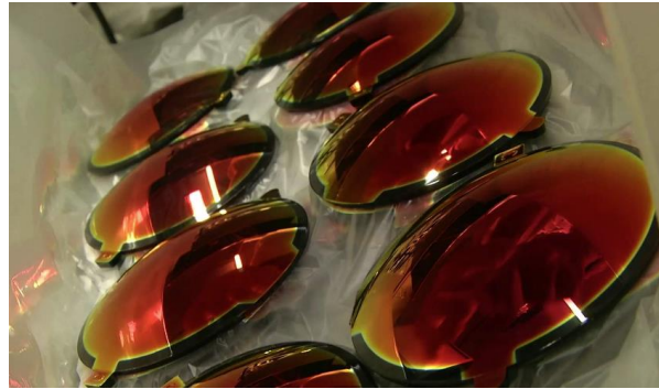
Image 1.3.6 - Luxottica's Plastic Lenses production presentation (2022). "Solid Mirroring coating on plastic meniscuses". Leonardo, Science for a new Vision
