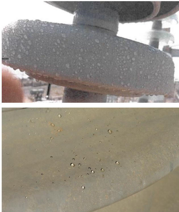
Figure [13]. Hydrophobicity of coated glass and ceramic insulators.
