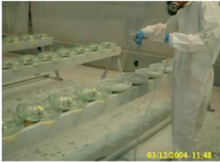
Rendina, R., et al. "First experience with factory coated glass insulators on the italian transmission network.", 2007.
