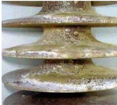
Figure [8]. Grease oxidation
