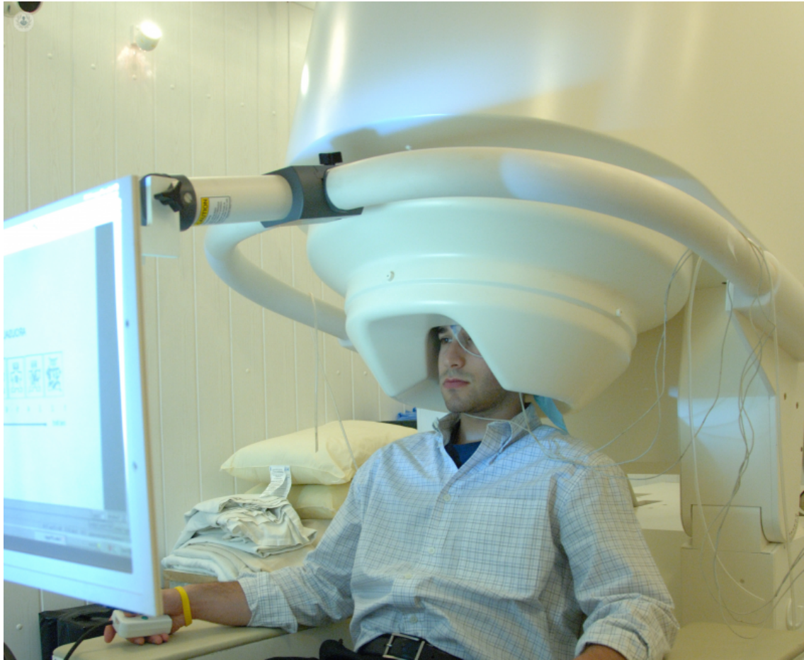
Figure 9: a MEG machine used for measuring magnetic fields generated by neural activity
