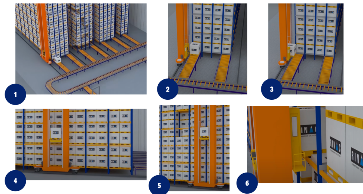
Figure 55 - Step-by-step operation of an automated storage and retrieval system (AS/RS)
