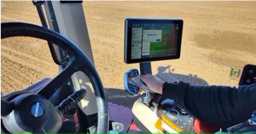
Figure 6: Displays mounted on self-driving tractors that allow the operator to view and follow trajectories plotted on prescription maps. Photo Source Il Sole 24 Ore
